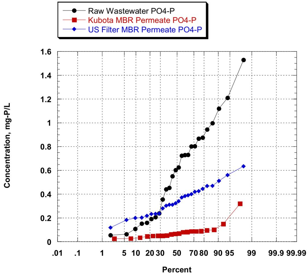
Figure 8-5 Probability Plot of Phosphate Removal by MBR Systems during Phase I (Part 1)
