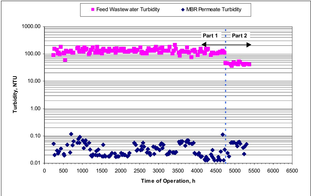
Figure 5-11: Turbidity Removal by the US Filter MBR
