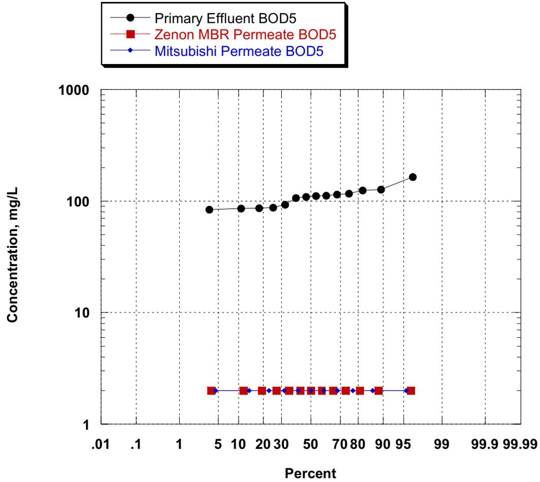
Figure 8-10 Probability Plot of BOD<sub>5</sub> Removal by MBR Systems during Phase II
