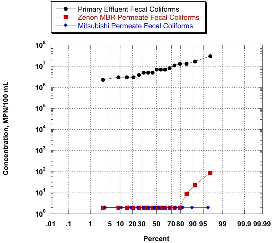
Figure 8-15 Probability Plot of Fecal Coliform Removal by MBR Systems during Phase II
