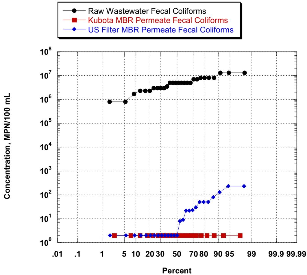
Figure 8-7 Probability Plot of Fecal Coliform Removal by MBRs during Phase I (Part 1)
