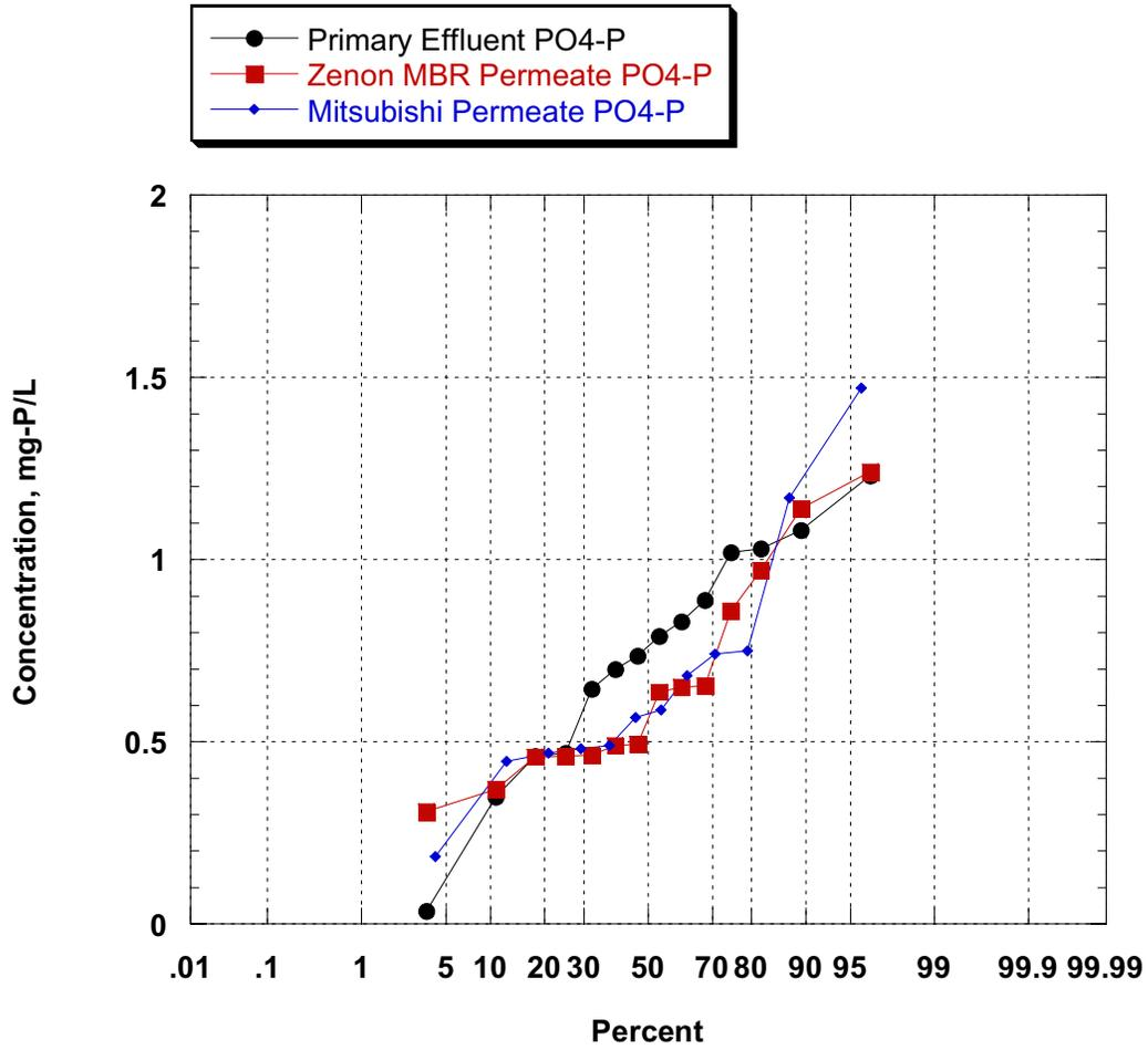
Figure 8-13 Probability Plot of Ortho-Phosphate Removal by MBR Systems during Phase II
