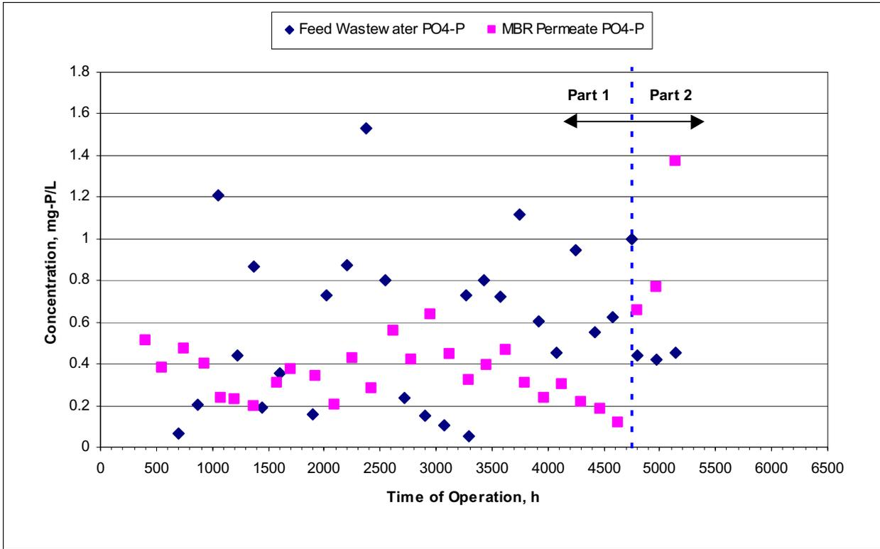
Figure 5-17: Ortho-Phosphate Removal by the US Filter MBR
