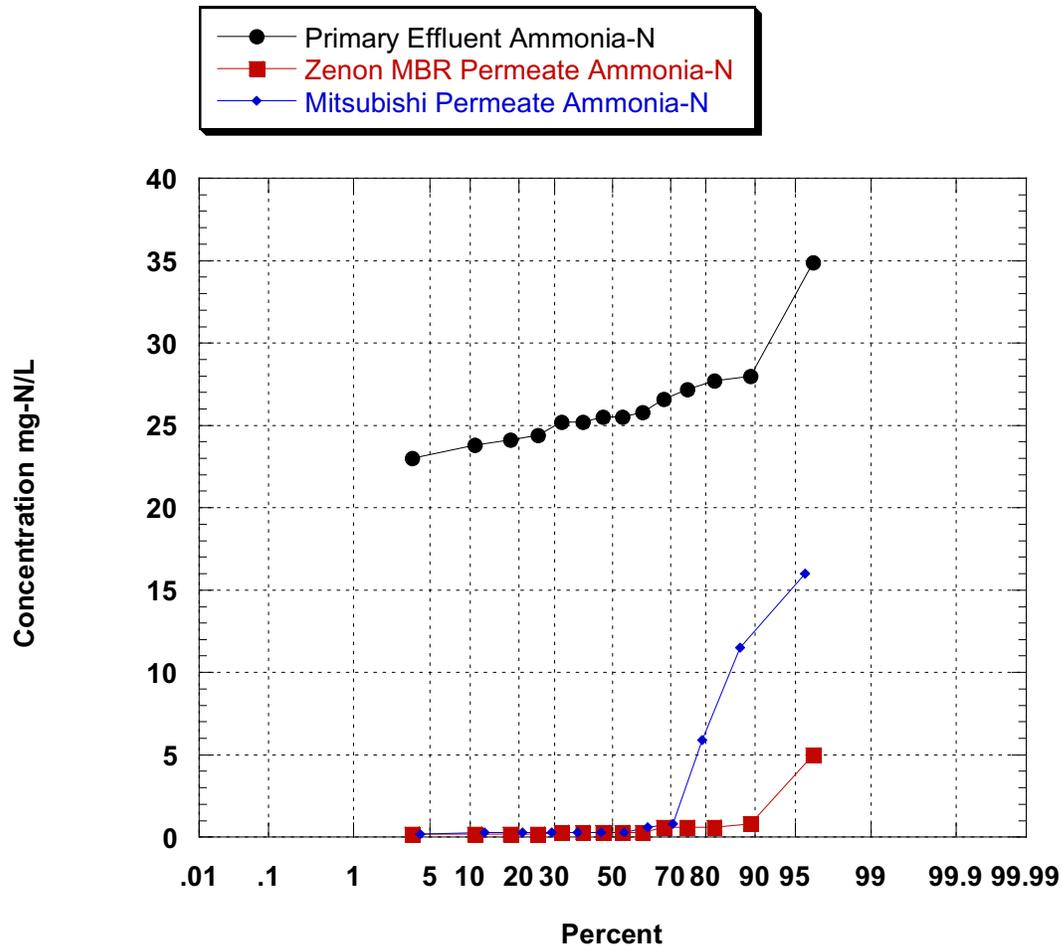
Figure 8-12 Probability Plot of Ammonia Removal by MBR Systems during Phase II
