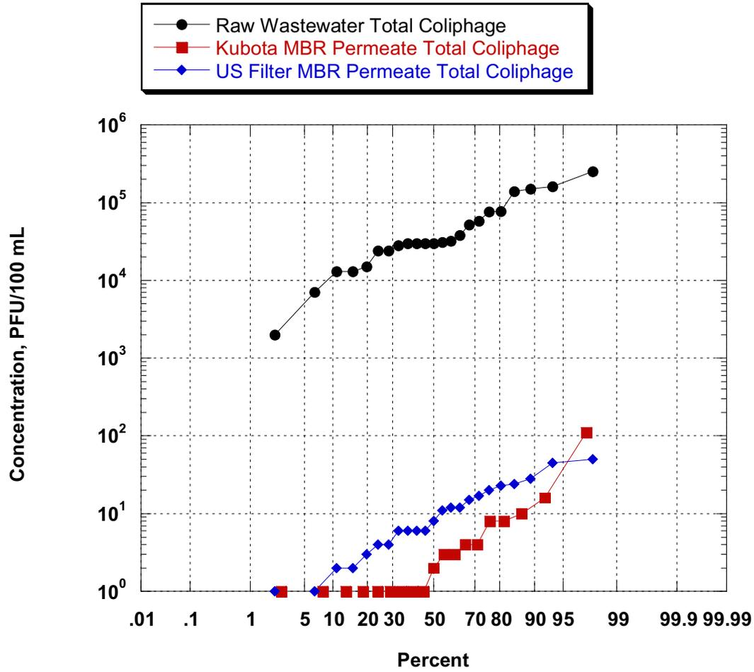
Figure 8-8 Probability Plot of the Total Coliphage Removal by MBRs during Phase I (Part 1)
