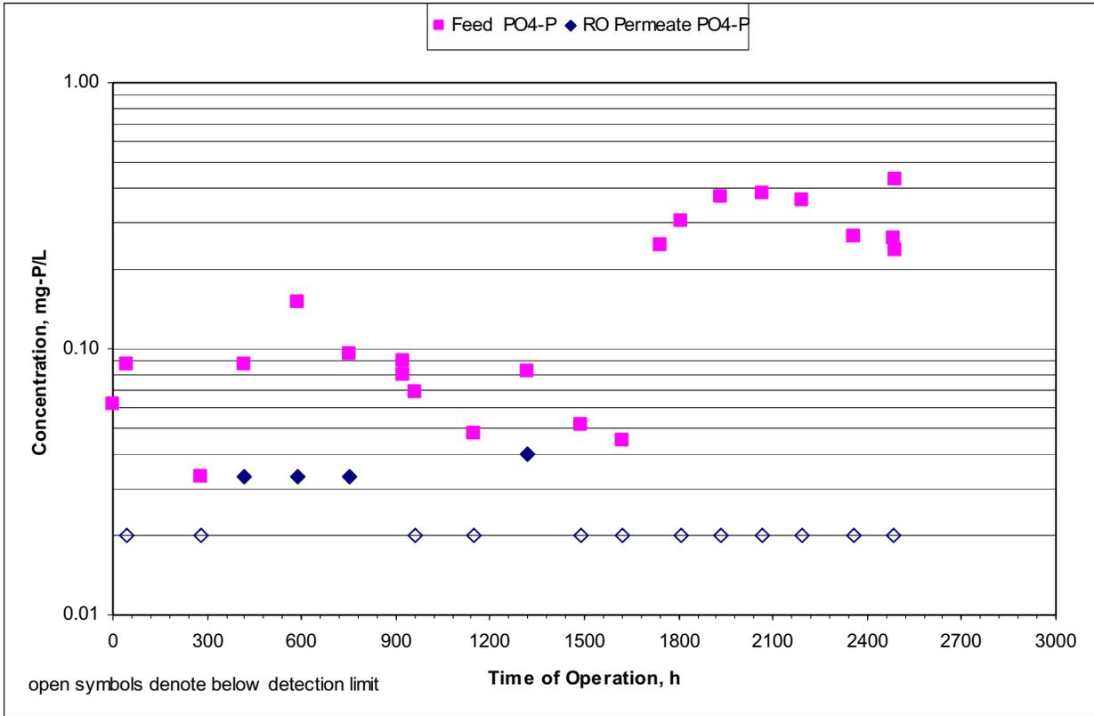
**Figure 5-24: Ortho-Phosphate Removal by the Hydranautics LFC3 RO Membrane**
