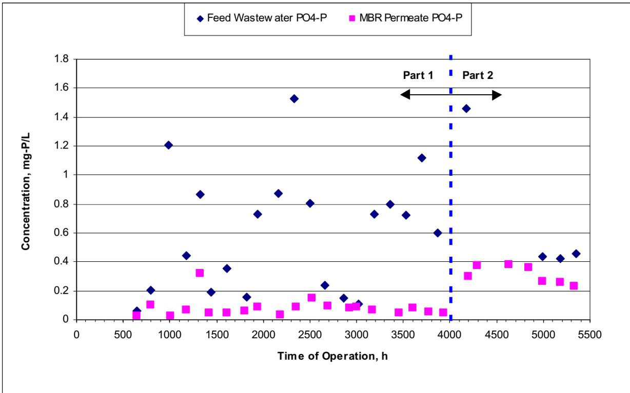
Figure 5-18: Ortho-Phosphate Removal by the Kubota MBR
