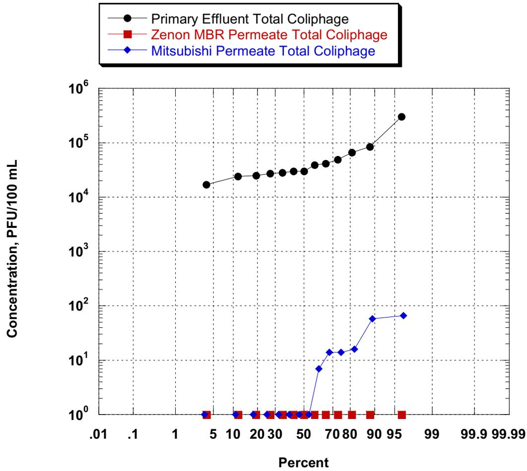
Figure 8-16 Probability Plot of Total Coliphage Removal by MBR Systems during Phase II
