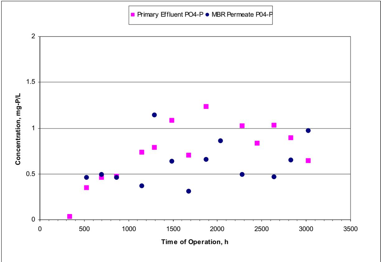
**Figure 6-15: Ortho-Phosphate Removal by the Zenon MBR**
