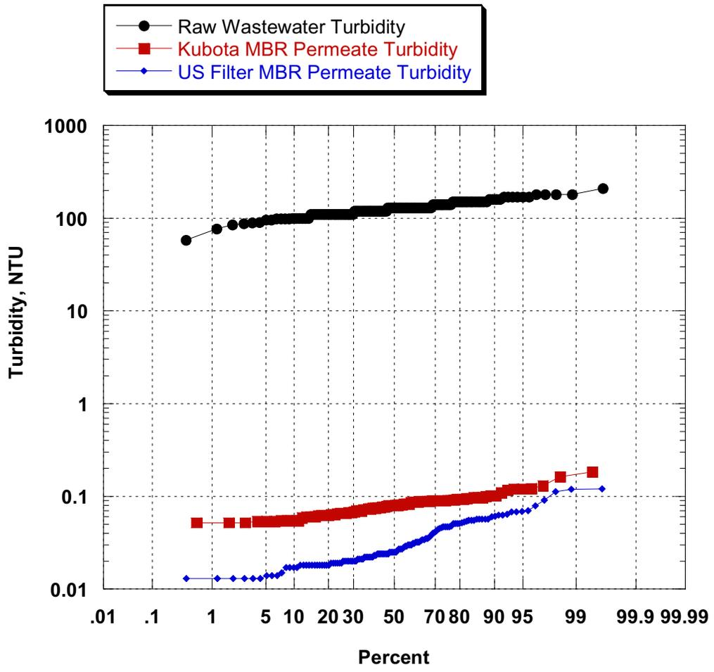
Figure 8-1: Probability Plot of Turbidity Removal by MBR Systems during Phase I (Part 1)
