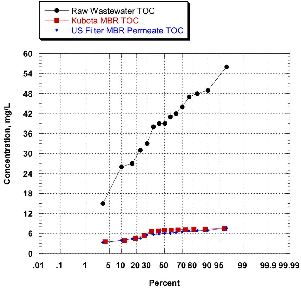
Figure 8-3 Probability Plot of TOC Removal by MBR Systems during Phase I (Part 1)
