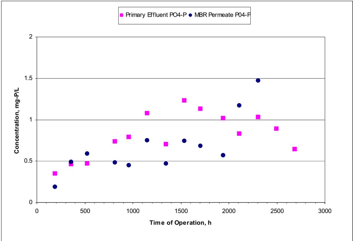
**Figure 6-17: Ortho-Phosphate Removal by the Mitsubishi MBR**
