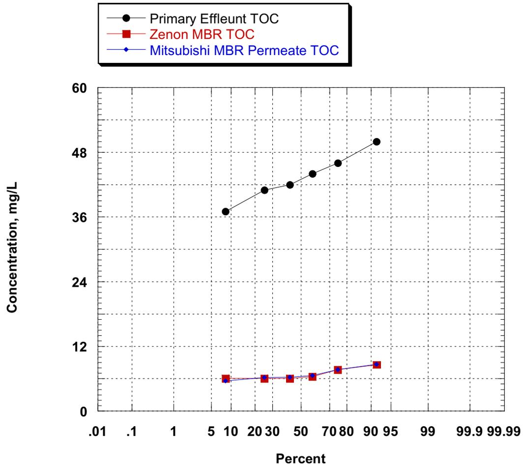
Figure 8-11 Probability Plot of TOC Removal by MBR Pilot Systems during Phase II
