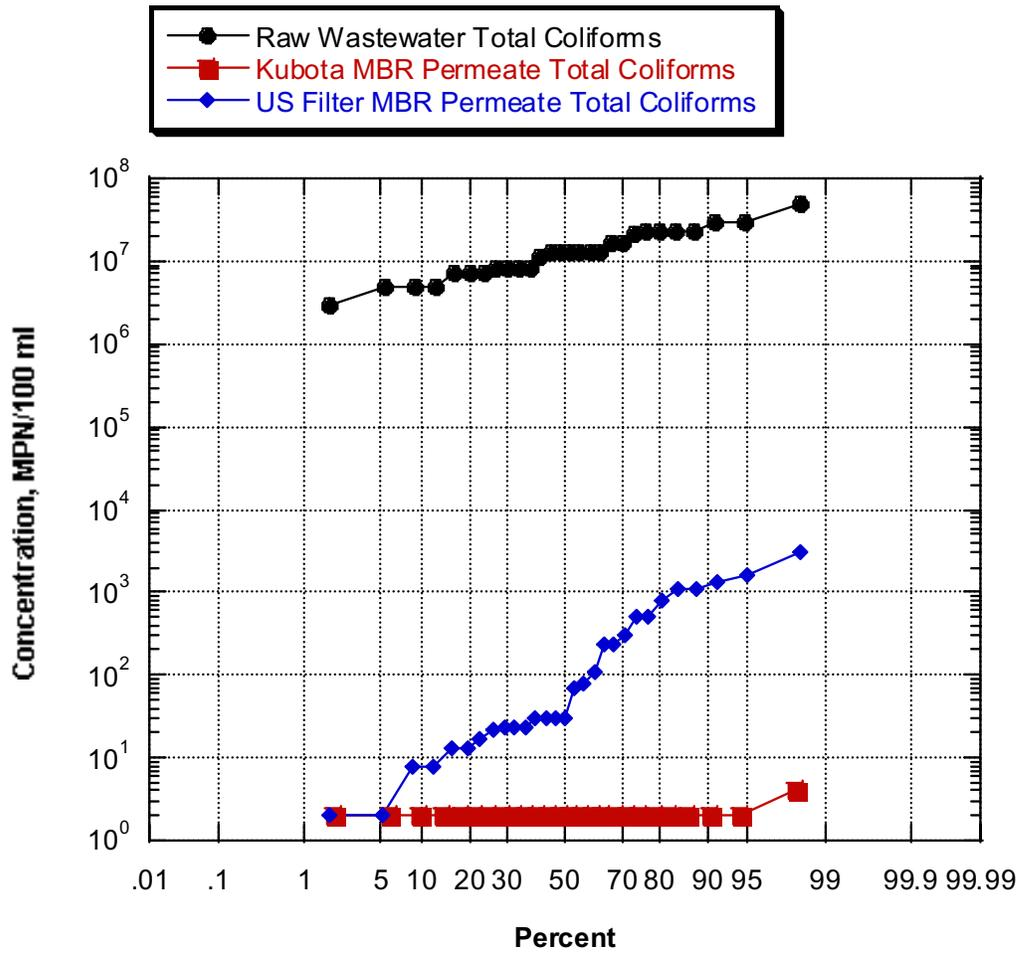
Figure 8-6 Probability Plot of Total Coliform Removal by MBRs during Phase I (Part 1)
