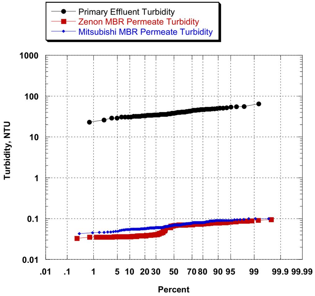
Figure 8-9 Probability Plot of the Turbidity Removal by MBRs during Phase II
