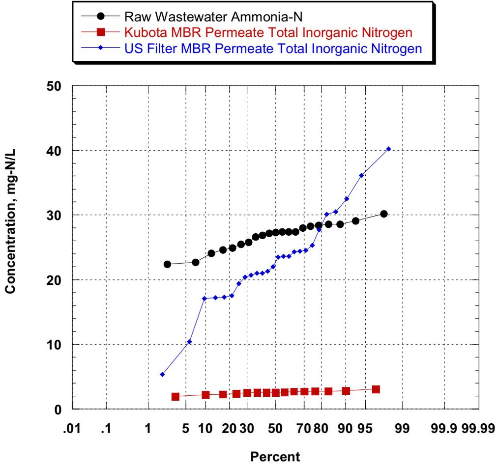
Figure 8-4 Probability Plot of Ammonia Removal by MBR Systems during Phase I (Part 1)
