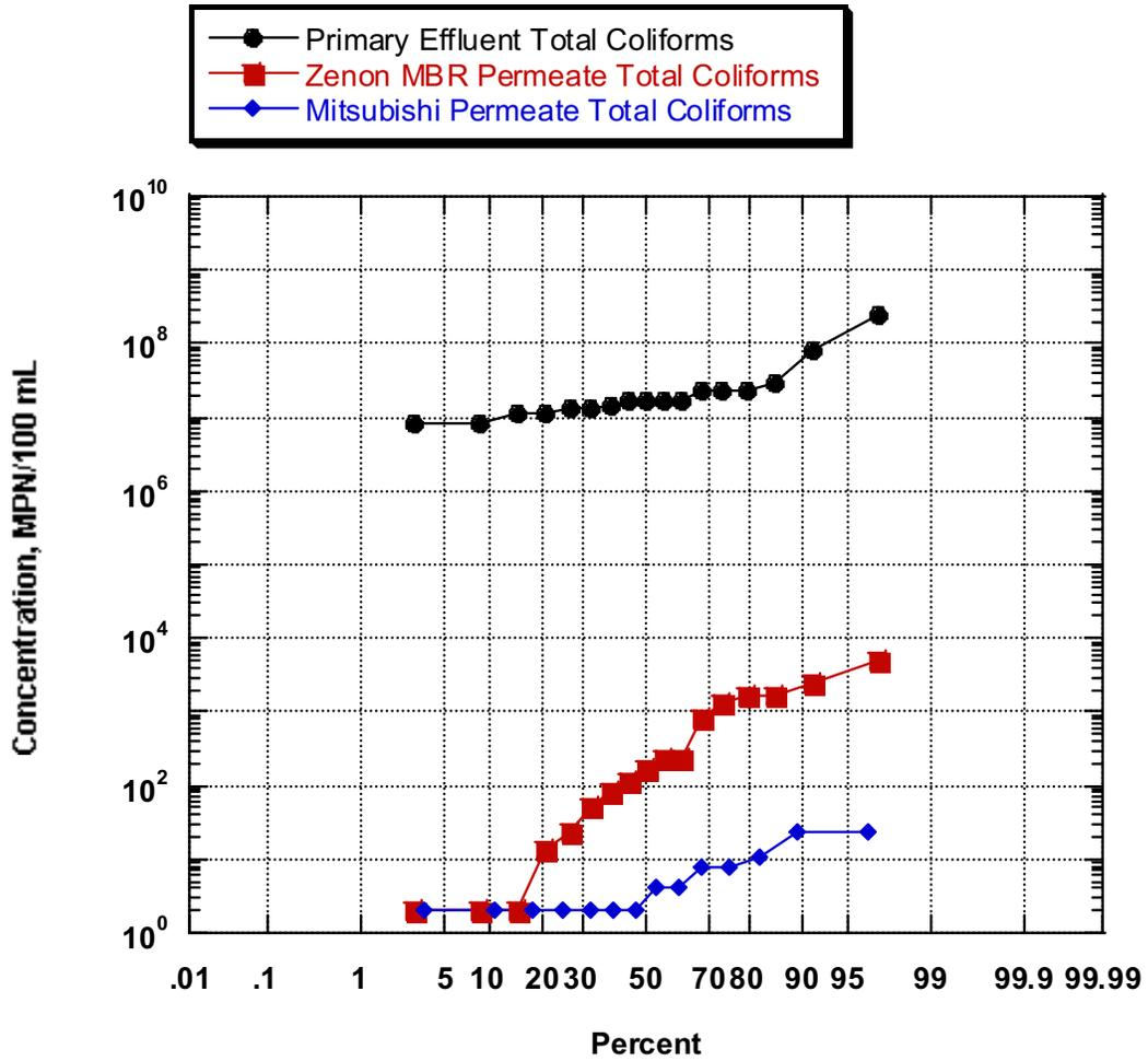
Figure 8-14 Probability Plot of Total Coliform Removal by MBR Systems during Phase II
