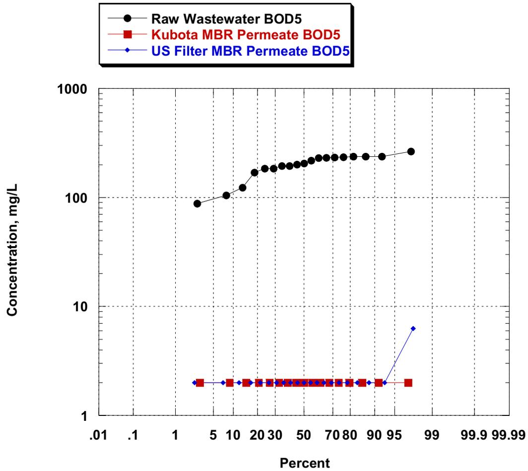
Figure 8-2 Probability Plot of BOD<sub>5</sub> Removal by MBR Systems during Phase I (Part 1)
