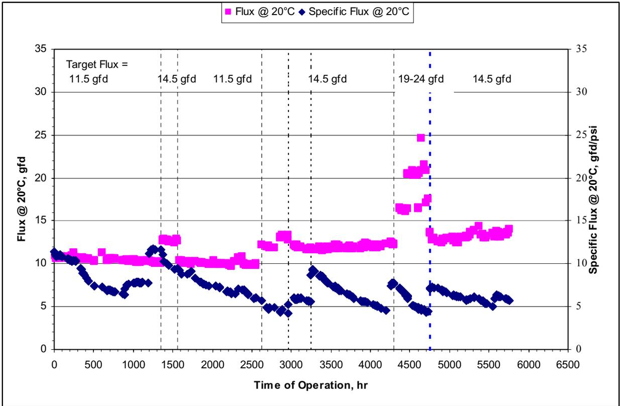
Figure 5-7: Membrane Performance of the US Filter MBR
